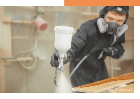
Paint has been used for thousands of years as a decorative, protective or functional additive to finished products. The application of paint using various air spray processes has become the norm. With these processes, comes a multitude of hazards. The major exposures associated with paint spray processes are fire, explosion and health hazards.
